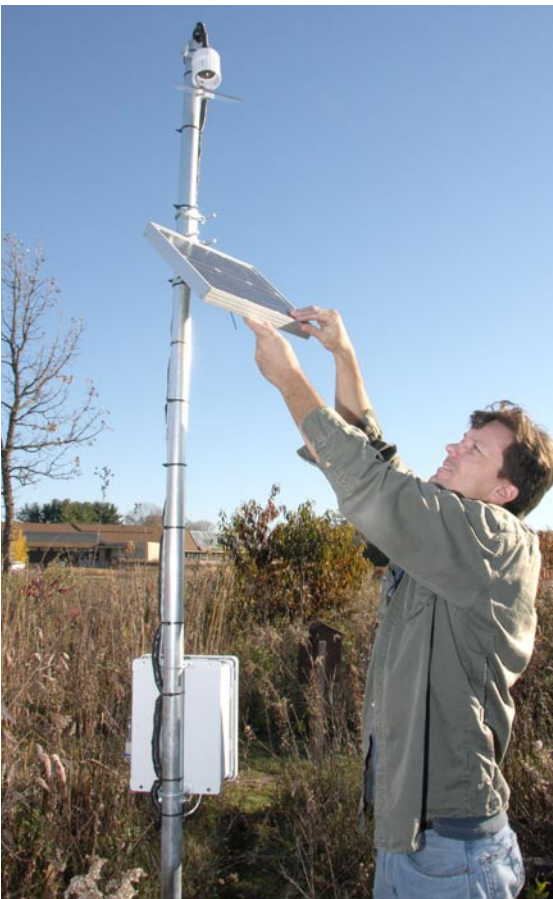
Bat Ecologist David Redell inspects the solar panel on the bat tracking station. This panel collects electrical energy from the sun during the day, which is used to power the audio gathering system when it automatically switches on in the evening. Photo by Bill Arthur
