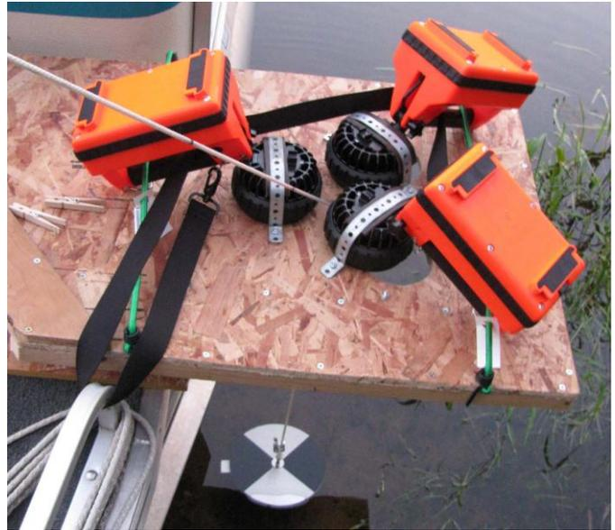
Figure 2 Lanterns mounted on platform with adjustable tilt.
