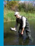
Laura De Galier, Park Watch Volunteer checks Dissolved Oxygen at Site #3 utilizing the VSI550A DO Meter.
