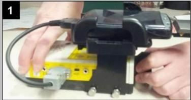
Firmly grasp the detector with one hand near the back of the detector and place one hand over the microphone.
