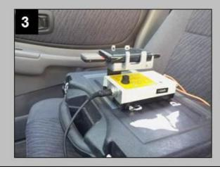
The detector should be placed in a secure position in the cab of your vehicle and be readily available so you can verify that the GPS is working properly throughout the survey.
