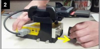
PULL the microphone straight back to remove. DO NOT turn or twist microphone as damage to the sensitive pins will occur.
