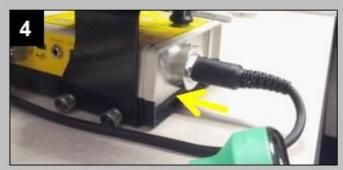
*PUSH* the cord directly into the detector it has firmly seeded.
