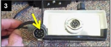
Align pins to fit by ensuring missing pin always matches the detector plug. The plug should easily insert into the detector.
