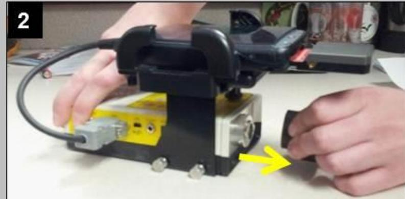
**2** *PULL* the microphone straight back to remove. **DO NOT** turn or twist microphone as damage to the sensitive pins will occur.
