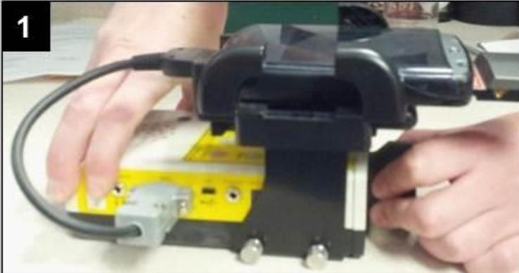
**1** Firmly grasp the detector with one hand near the back of the detector and place one hand over the microphone.
