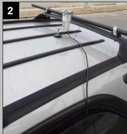
If possible, it is best to use a window that does not need to be open and closed, such as a passenger or rear door.
