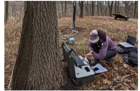
Setting up a PIT tag scanning antenna at a bat maternity roost in early spring before bats arrive for the summer. Photo by J. Paul White
