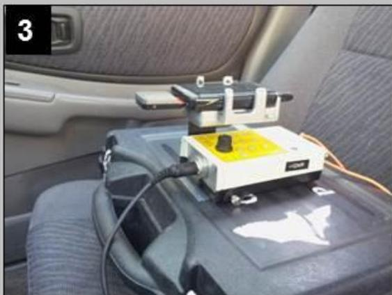
The detector should be placed in a secure position in the cab of your vehicle and be readily available so you can verify that the GPS is working properly throughout the survey.
