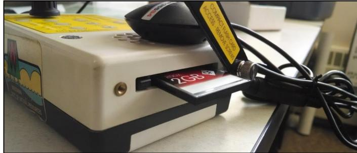
Step 2: Secure the GPS connection to the side of the detector (use two black knobbed bolts to secure cord to serial port of detector). The USB end will insert into power pack and GPS circular disc can be placed on back of the detector, secured by an internal magnet. Ensure the GPS has 2 charged AA batteries and the detector has 4 charged AA batteries.
