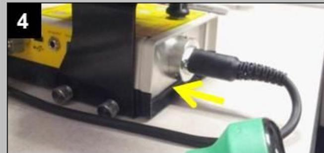
**4** *PUSH* the cord directly into the detector it has firmly seeded.
