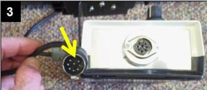
**3** Align pins to fit by ensuring missing pin always matches the detector plug. The plug should easily insert into the detector.
